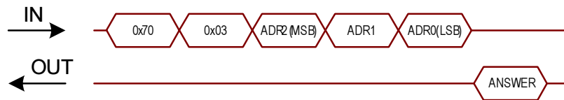
Figure 21: Flash-memory data read command
