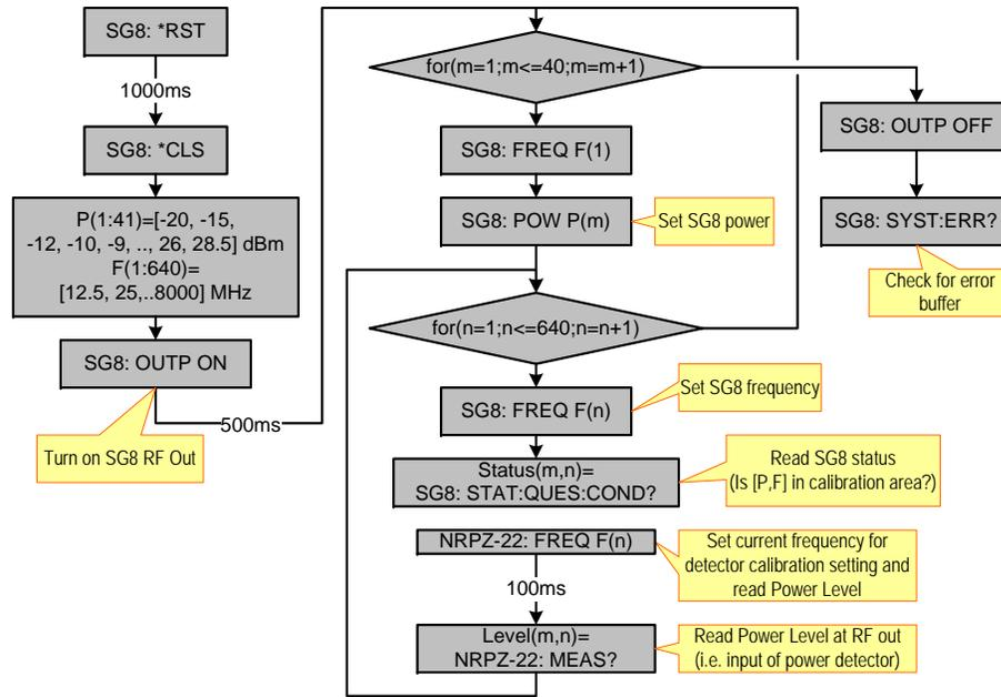
Figure 5: SG8 Level Scan algorithm
