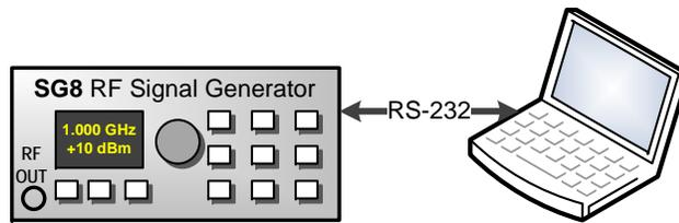
Figure 3: RS-232 Test Setup
