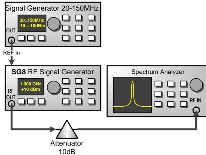
Figure 10: REF In sensitivity test setup
