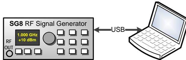
Figure 2: USB Test Setup
