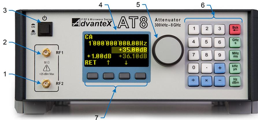
Figure 3: Front panel view
