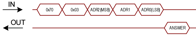
Figure 21: Flash-memory data read command
