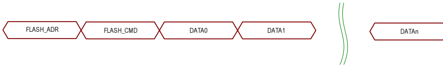
Figure 20: Structure of flash-memory data transfer
