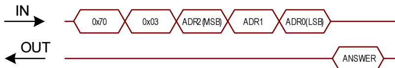
Figure 26: Flash-memory data read command
